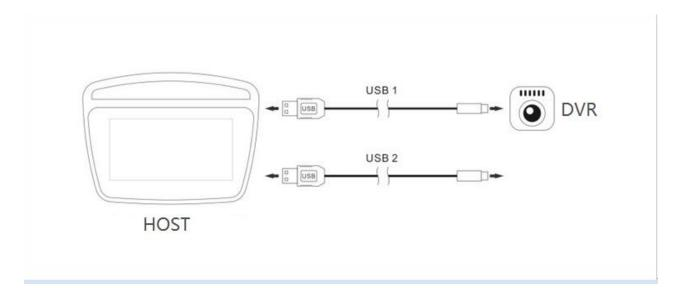
\*Notes: Normally choose the random USB interface of the large screen host machine for connection, e.g. USB1. Replace USB2 interface if the equipment cannot be normally found.
